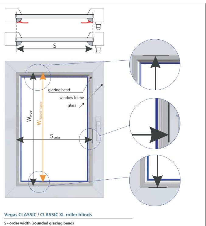
Give the width of the external edges of the glazing beads.
